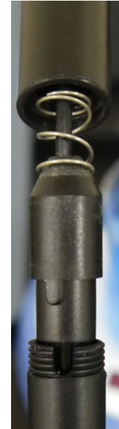
Ammonia ISE is spring loaded to refresh fill solution around the pH electrode
