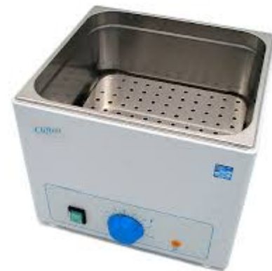
Water bath 44.5 \pm 0.2^{\circ}\text{C}
