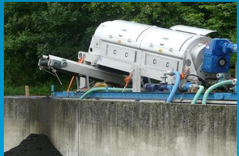
Screw Press Image Courtesy of Huber Technology, Inc.
