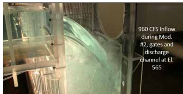
Figure 5: Model showing no overflow after implementation of Modification #2
