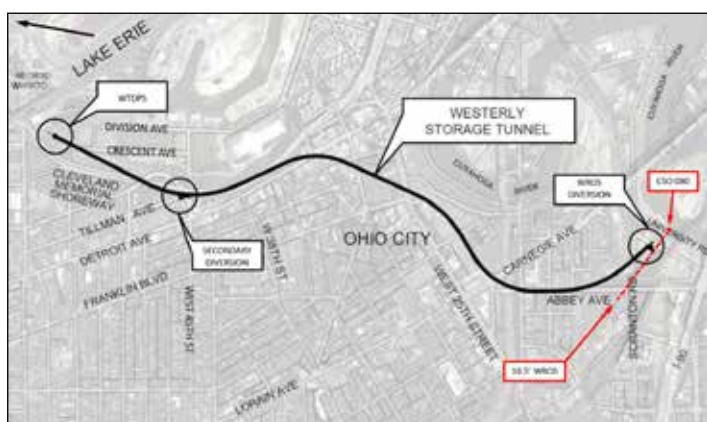
Figure 1: The WST Alignment, flowing from the WROS Diversion Structure down to WTDPS and ultimately the WWWTC
