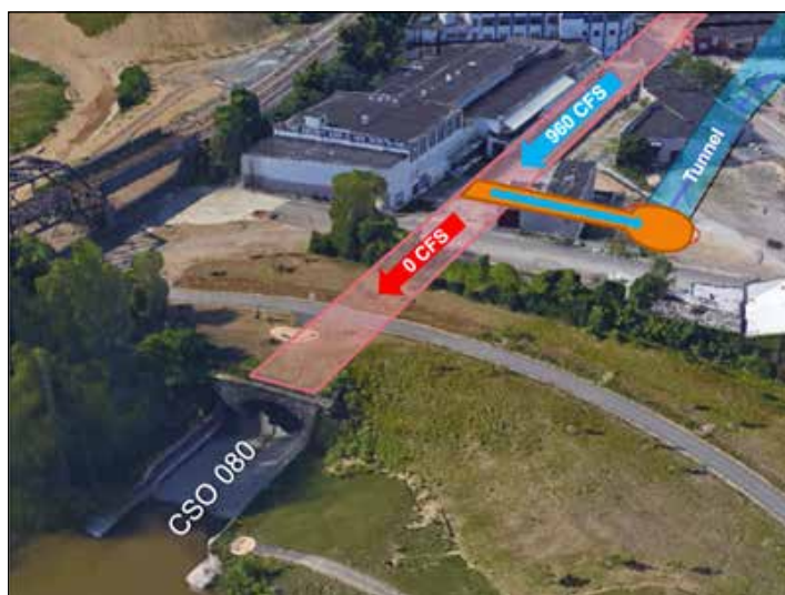
Figure 2: Schematic view of the WROS Diversion
