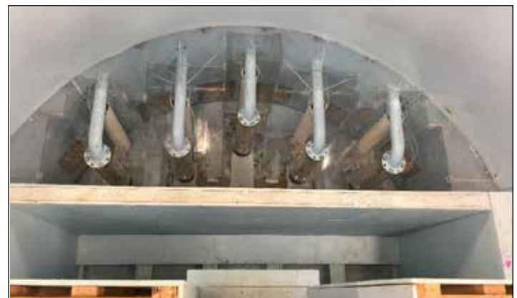
Figure 7: WTDPS wet well geometry as represented in the physical model
