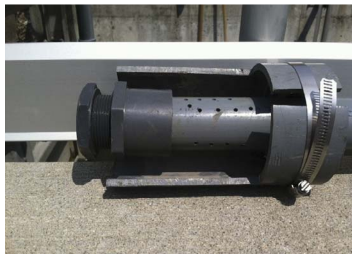
Figure 1: These pictures show the PVC pipe used as a pre-filter (Left) and the end of the pipe with the 1/8 inch holes and rag shield. (Right)
